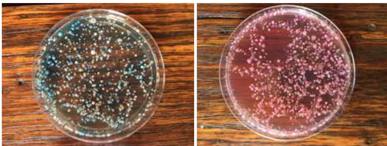
Blue and red agar in petri dishes clearly showing the presence of E. coli and faecal coliform bacteria in the 2019 water tests.
