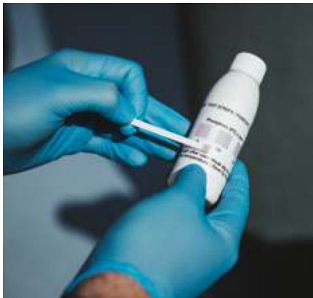
One of the tests conducted by AfriForum involves test strips to test phosphate levels in water.
